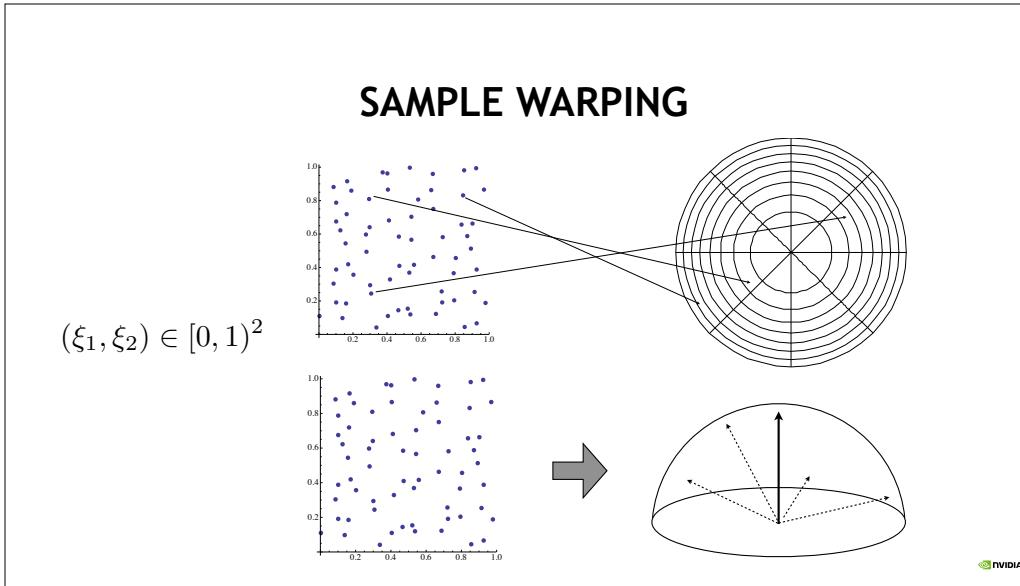
All of these sampling techniques are based on warping random numbers from the unit square to some other domain—to the hemisphere, to the sphere, to the cone surrounding a sphere, to a disk. You can also generate samples from a BSDF's scattering distribution, or choose directions to an IBL light source.
