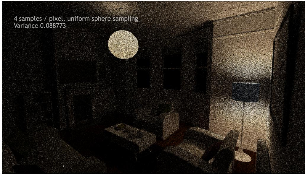
Let's see how that works out for us. Here's a scene with two spherical light sources, rendered with 4 rays per pixel, sampling points on the entire sphere.
