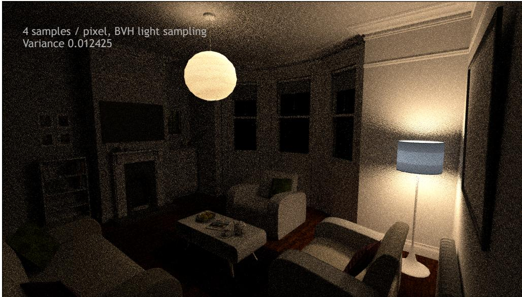
Here's the scene rendered using Sony's light sampling technique. Variance is 2.46x lower! Look at the difference on the wall by the light with the blue shade, for example—there you're close to that light, and the other's making a relatively small contribution. It's not worth tracing so many rays to it.
