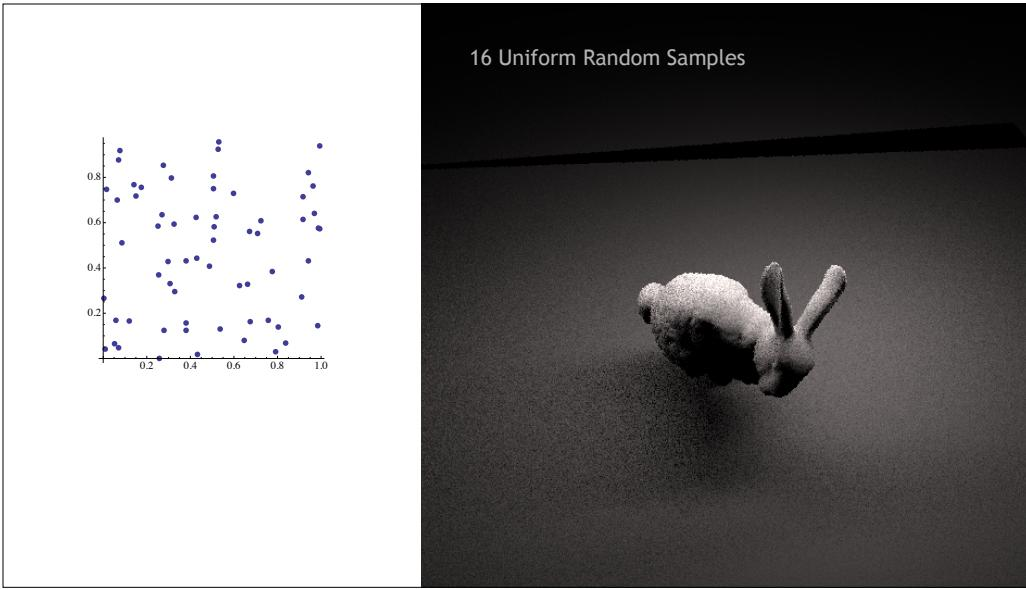
Here is a plot of 64 random samples and then an image rendered with 16 random samples per pixel. There's a long skinny triangle area light illuminating the bunny—you can see the black back side of it above the bunny.
