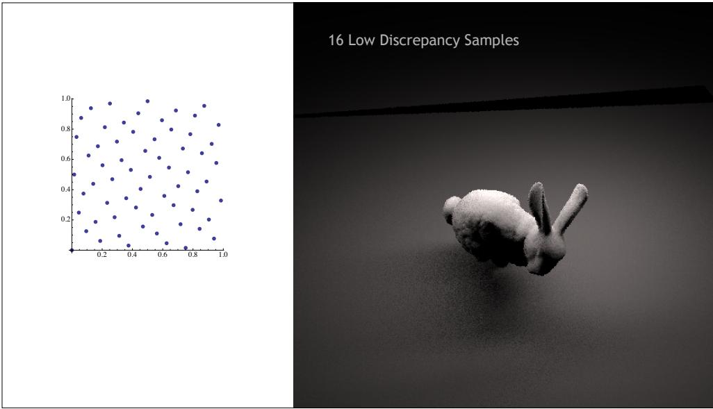
Here's that scene rendered with this sampling pattern. It's not random. You can see a nice structure to the samples—they're not clumped together. You can see that the image is cleaner for the same number of rays.
