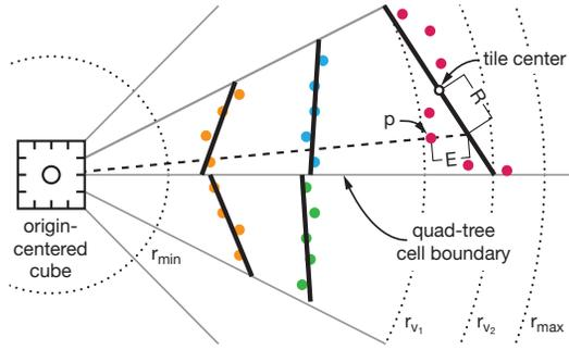
Fig. 4. The energy term  $E(p, t)$  (Equation 2) models the error in approximating a scene sample point  $p$  with the quad  $t$ .
