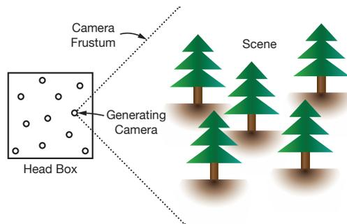
Fig. 3. The scene is captured by rendering RGB and depth cube maps from a set of view points inside the viewing region.
