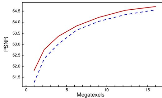
Fig. 14. PSNR of rendered images as a function of texture atlas size for the SMITHY scene when using content adaptive texturing (solid red line) and not using it (dashed blue line). For this scene the number of texels may be reduced by 57, 30, 21 and 18 percent for an initial atlas size of 1, 4, 9 and 16 megatexels, respectively.
